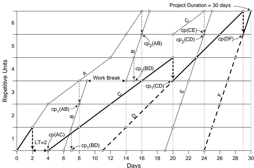
FIG. 7. RSM Diagram for a Six Unit Project
