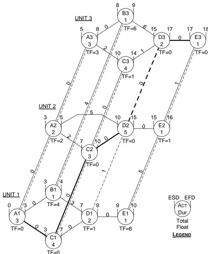
FIG. 1. CPM Network for Three Repetitive Units
